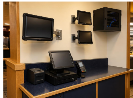
POS terminal, card reader, receipt printer, kitchen display and bump bar.
