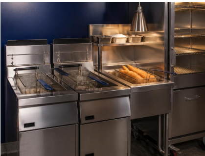
Fry line: twin-vat fryers, filter cart clearance, dump and crisping station.
